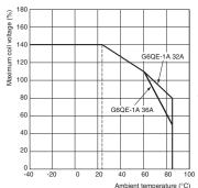
Connecting Method: Mounted 3 Relays horizontally based on **EN Standards** Installation Interval: 50 mm
