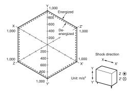
Conditions: Shock is applied in ±X, ±Y, and ±Z
